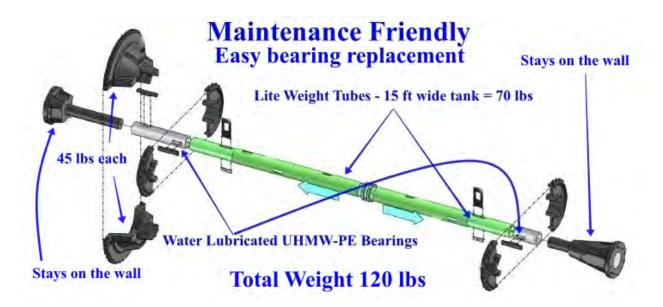
45° Biaxially wrapped FRP telescopic tube assembly Lite Weight while being able to withstand 58-60,000 in-lbs. of torque Replaceable UHMW Bearings – water lubricated Non-Corrosive – doesn't lock up even when dry for days Maintenance friendly – 3-4 hours to completely replace bearings Mounting spindles - non-metallic Cast Nylon. Structurally sound after 30 years of service
